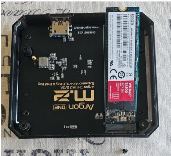
Slot the SSD within the connector with an angle (30 degrees)
