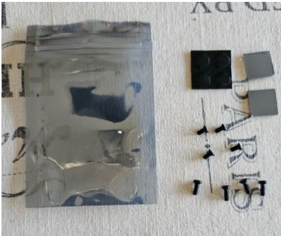
Screws, thermal pad and rubber feet included in Argon M2 case package.
