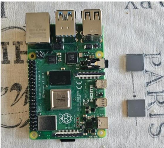
The thermal pads need to be seated on the board chipset.
