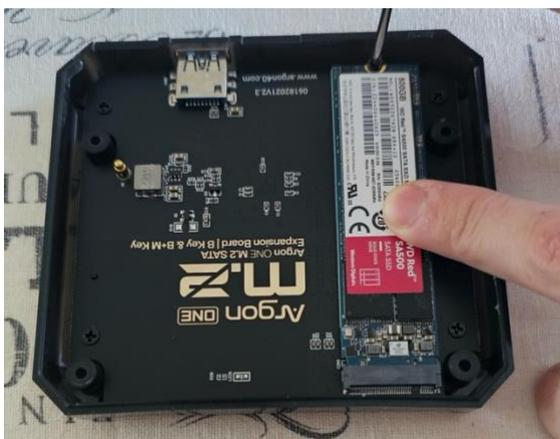
Push the SSD to the horizontal and lock it with the dedicated lock screw
