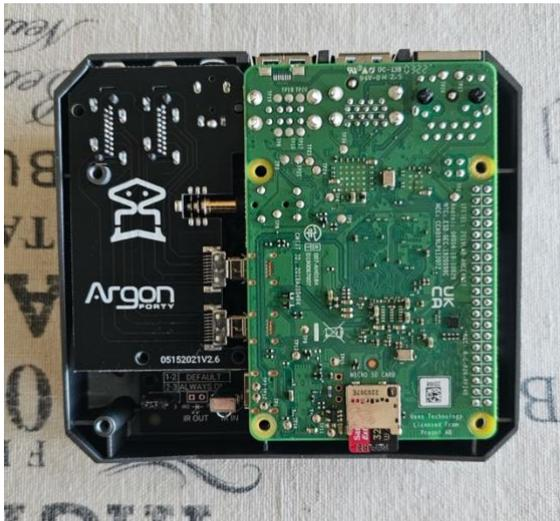
Use shorter flat head screws to fasten Raspberry Pi and HDMI board assembly to the top case.
