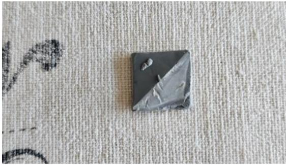
On both sides of the thermal pad, remove the plastic.
