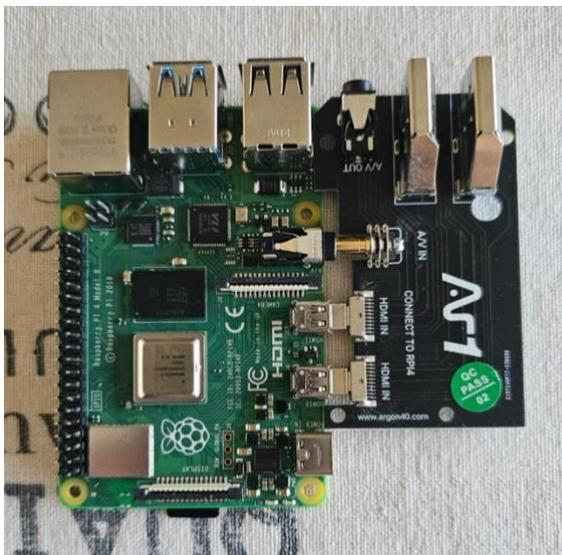
Connect Raspberry Pi to Argon HDMI board
